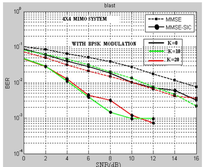
Fig: 3 BER Vs SNR curve for 4X4 MIMO system with different K for MMSE and MMSE-SIC receiver.
