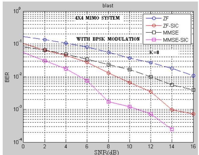
Fig: 2 BER Vs SNR curve for 4X4 MIMO system with different receiver.
