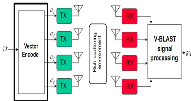
Fig. 1. Block diagram of BLAST system.
