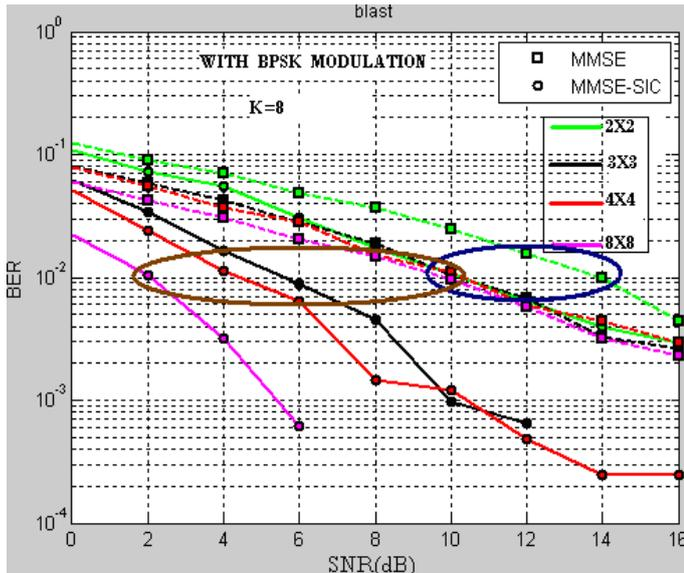
Fig: 4 BER Vs SNR curve for Different MIMO system for MMSE and MMSE-SIC receiver (with K=8).
