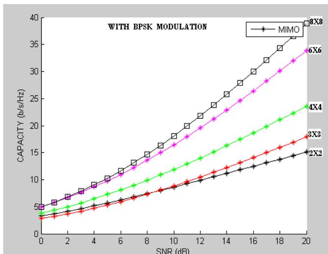
Fig: 1 CAPACITY Vs SNR curve for different MIMO system.
