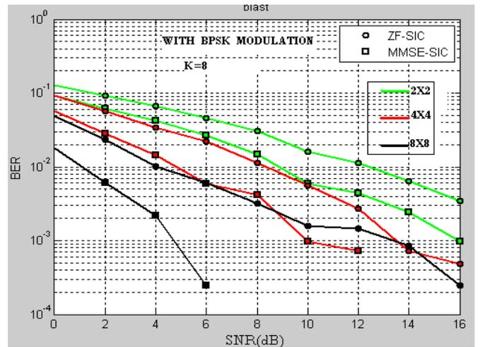
Fig: 5 BER Vs SNR curve for Different MIMO system for MMSE-SIC and ZF-SIC receiver (with K=8).
